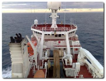
Árni Friðriksson is built as a multipurpose research vessel, designed for oceanographic and fisheries research in temperate and artic waters (LR Ice Class 1B on the hull). The propulsion system is of diesel electric type to secure low noise levels. The vessel is equipped with sophisticated electronic equipment for stock assessment, bottom mapping and communication.
